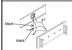
Make wiring connections, black wire from fixture to black wire from junction box. white wire from fixture to white wire from junction box.
