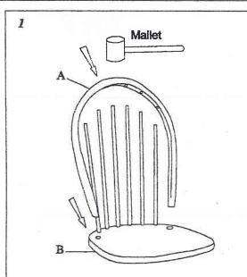
Fix the Spindles (D),(E) & (F) to the Hoop (A) & seat (B) , use a mallet to knock the spindles fit in the holes
