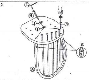
Place the assembled chair seat on a soft and fiat surface to prevent scratches. Insert JRN Nut (K) into holes on hoop (A) and assemble hoop (A) using JCBC Screw (H), Spring Washer (J) and Flat Washer (I) in line with JRN Nut (K). Please tighten JCBC Screw (H) With Allen key (L), then assemble spindles (D), (E), (F) with chair seat by JCBC serew(N)
