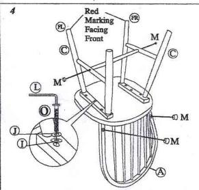
Attach the Leg Frame (C) to the Chair Seat (B). Red Marking on leg frame shoud facing front, Secure it using JCBC (O) Spring washer (J) and Flat washer (I) Tighten it with Allen key (L). Insert the Wood Button (M) to the cover the hole on leg frame (C) & Hoop (A)
