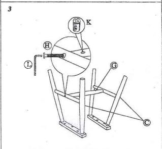
Assemble leg frame (C) and Crossbar (G) together by insert the JRN Nut(K) in the Crossbar (G), Secure using JCBC Screw (H) as shown.
