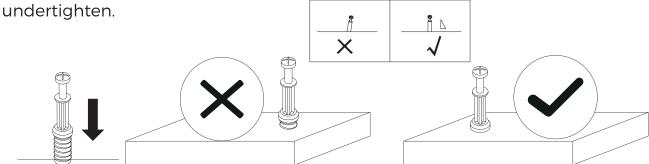
•When fitting cam lock, ensure starting position is correct beforeyou insert connecting quickfit.
