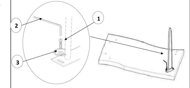
Place Leg(B) on the Table Top (A) as shown in the picture. Fix the Leg (B) using Long Bolt (1) and Washer (3) with the help of Allen key(2). Repeat the step and the attach the other Legs (B) on the Table Top (A). **DO NOT FULLY TIGHTHEN BOLTS.**
