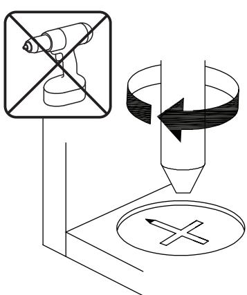
**EN**\_Turn cam lock clockwise to tighten.
