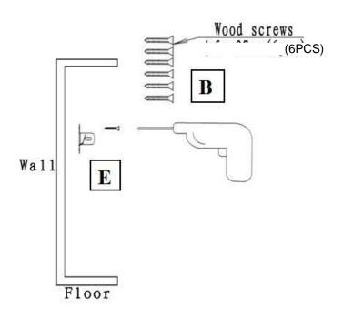
**STEP 3**) Have two people lift the fireplace machine up and insert the slots (2 slots on back of fireplace box) to the wall bracket hooks.
