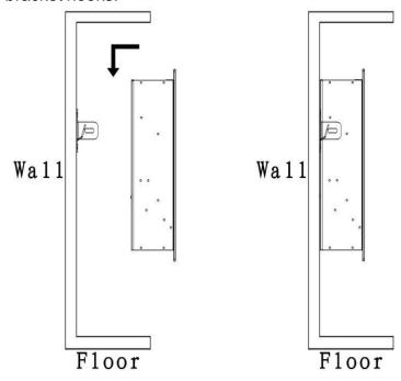
**STEP 4)** With the fireplace installed safely, then using screws driver to lock the bracket and fireplace with two ST4x8 (**D**) screws in both sides. Check the appliance for stability ensuring that the appliance will not pull free from the wall.
