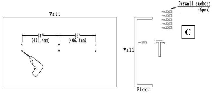
**STEP2**) Using the six wood screws (B) to fix the wall bracket, with wood screws thread the wall bracket and to lock with the drywall anchors, please tighten all wood screws.
