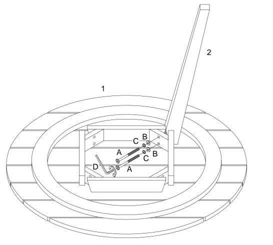
Fasten part (2) to part (1) by using bolt (A) with lock washer(C) and flat washer(B) with hex key (D)
