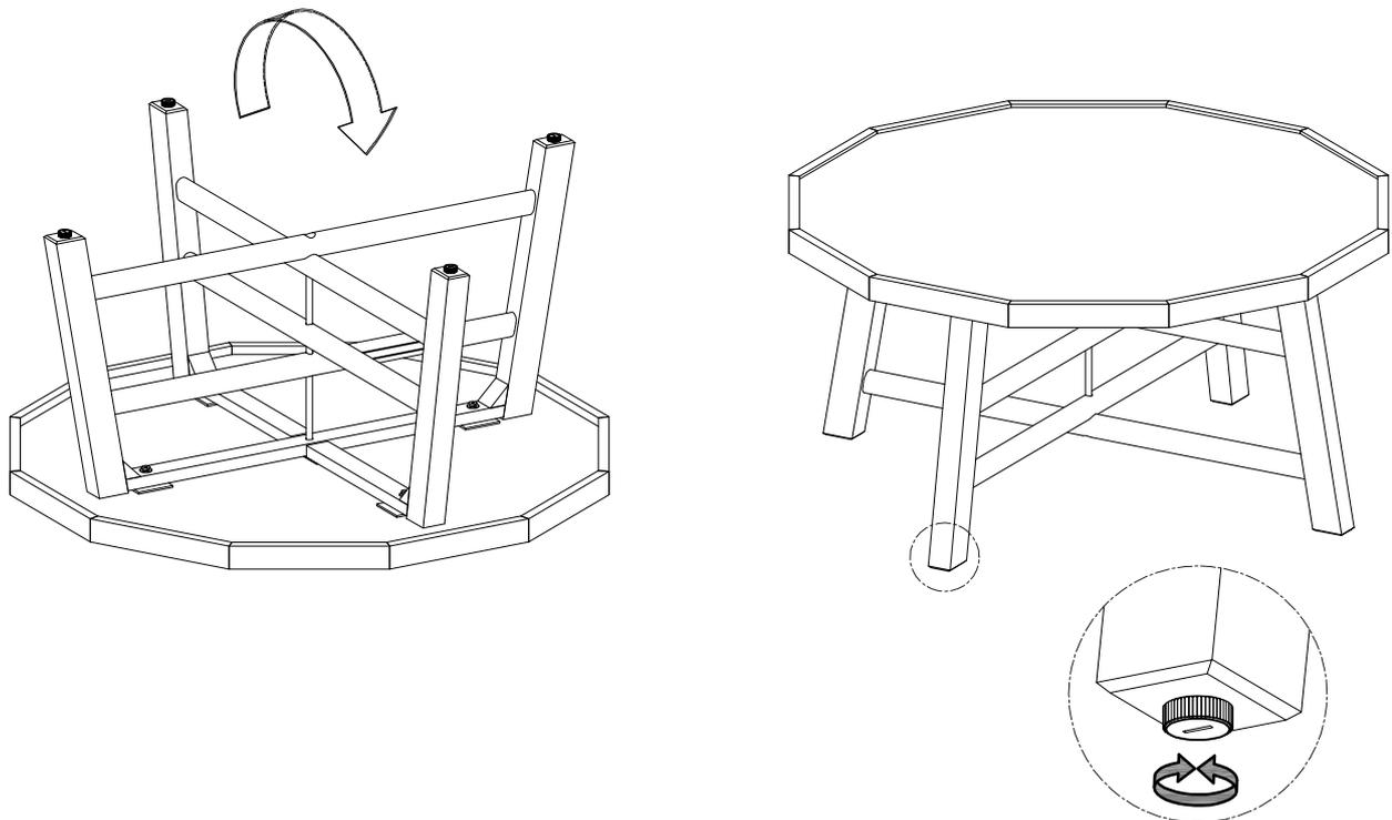
Note: adjust levelers on an uneven floor.
