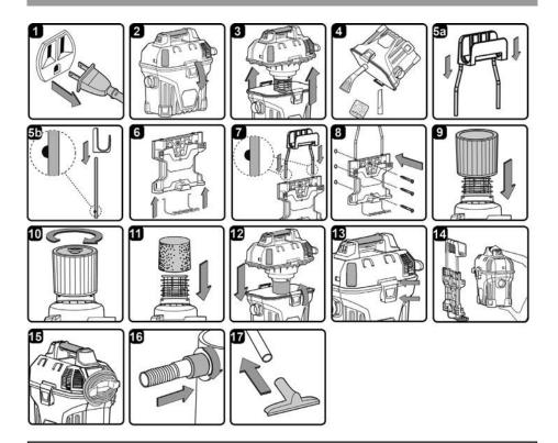
WARNING: TO REDUCE THE RISK OF ELECTRIC SHOCK - DO NOT EXPOSE TO RAIN. MAKE SURE PLUG IS DISCONNECTED BEFORE ASSEMBLING THE WET/DRY VAC.
