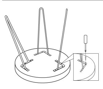
Attach the legs with the screws provided. Please note that the screws provided are the proper length for 1.5" to 2" thick.
