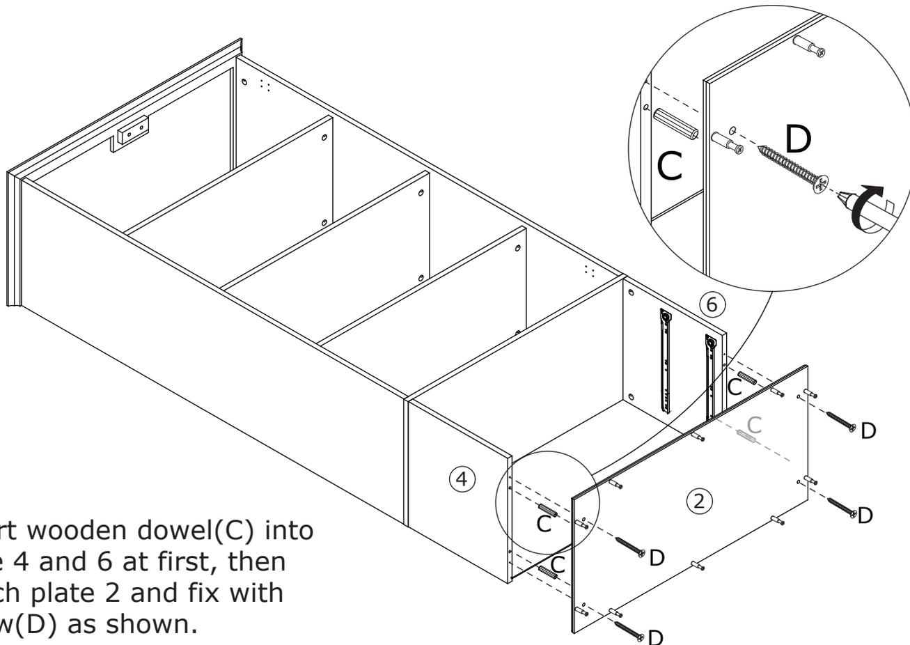
Insert wooden dowel(C) into plate 4 and 6 at first, then attach plate 2 and fix with screw(D) as shown.
