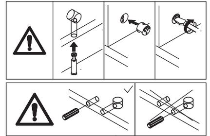
Put cam lock(B) into plate 3,5 and turn clockwise to tighten as shown.
