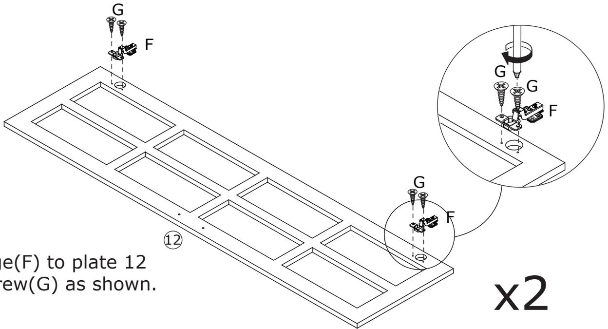
Fix hinge(F) to plate 12 with screw(G) as shown.
