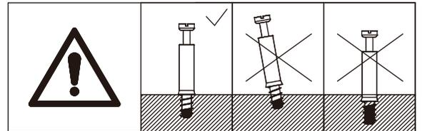
Insert quickfit screw(A) into plate 1 with a screwdriver as shown.
