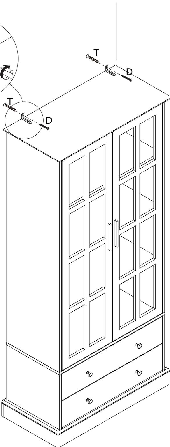
Install anti-tipping device as shown.
