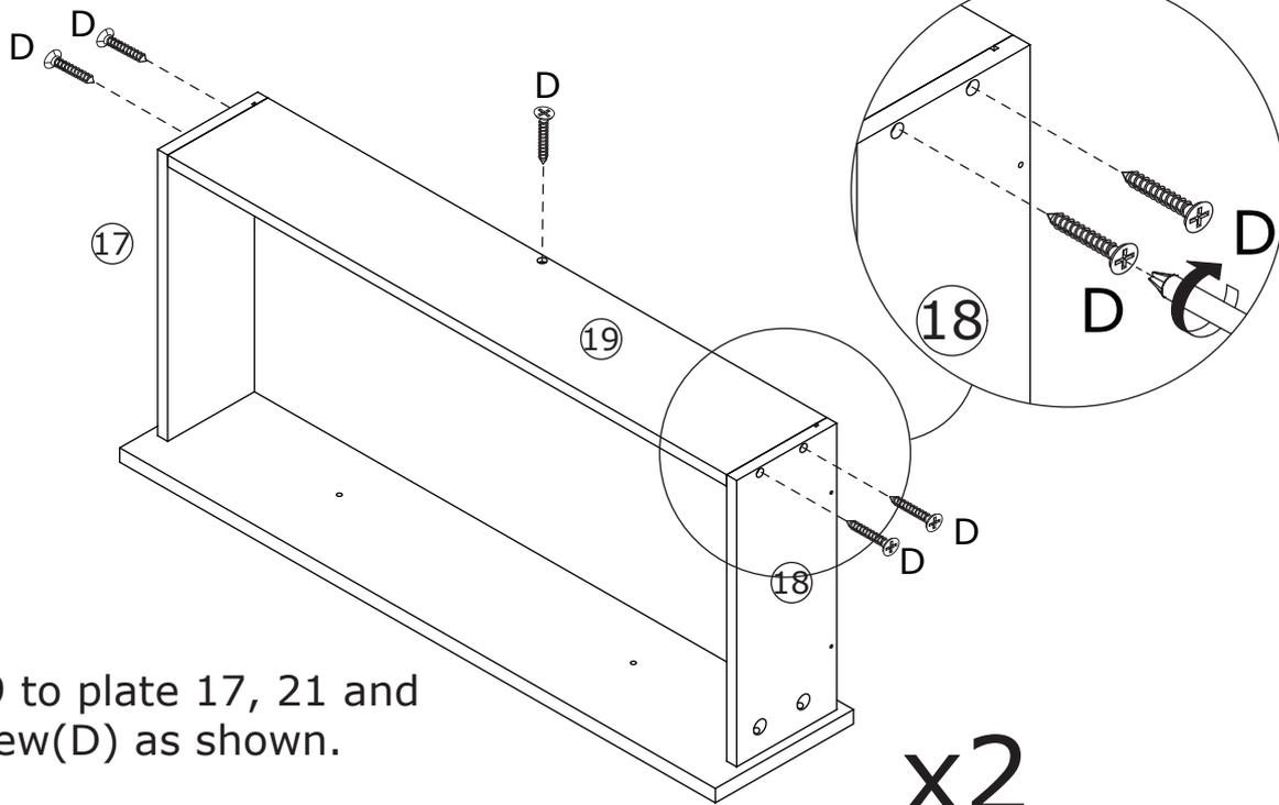
Fix plate 19 to plate 17, 21 and 18 with screw(D) as shown.
