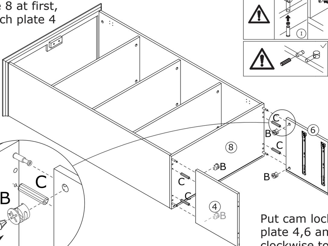
Put cam lock(B) into plate 4,6 and turn clockwise to tighten as shown.
