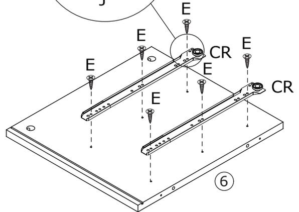
Fix slide rail(CL) and (CR) to plate 4 and 6 respectively with screw(E) as shown.
