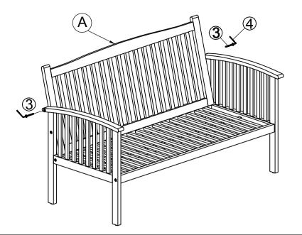
Use Bolt (3) with Allen Wrench (4) to affix the top of the Backrest to the Armrests on both sides as shown.
