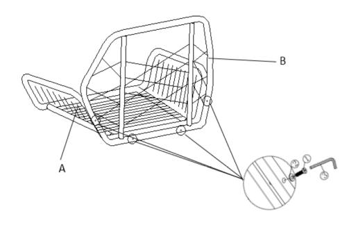
Open the carton and place all the parts onto a clean, non-marring surface. Align the Backrest(B) with Seat (A),
