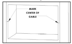
Align the Mounting Brackets with the mark keeping it flush against the gable.
