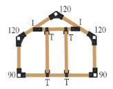
Please note: When assembling make sure brackets are facing the directions shown in this diagram.
