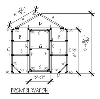
**Step 9:** Finally – measure your structure to determine the amount of materials you will need to purchase to cover your structure. Always make sure you allow for seams or waste material and purchase extra. To determine the amount of material needed for the front and rear of the structure measure the base for your width and then measure from the base to the top of the ridge for your height.
