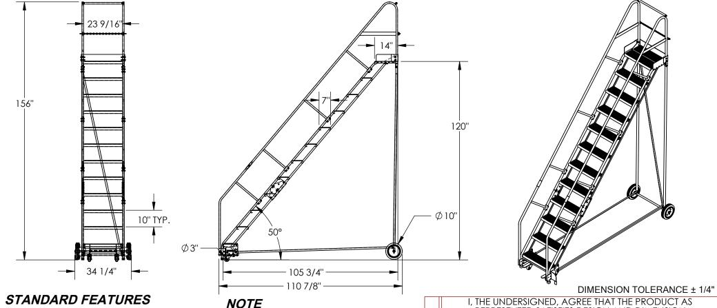
MODEL NUMBER IS LAD-12-14-P-EZ OVERALL WIDTH IS 34 1/4" USABLE WIDTH IS 23 9/16" **OVERALL LENGTH IS 110 7/8"** USABLE LENGTH IS 105 3/4" **OVERALL HEIGHT IS 156"** TOP STEP HEIGHT IS 120" STEP TYPE IS PERFORATED CLIMB ANGLE IS 50° STEP DEPTH IS 7" TOP STEP DEPTH IS 14" MAX CAPACITY IS 350 LBS WHEEL SIZE IS Ø10" FRONT WHEEL SIZE IS Ø3" TOUGH BAKED IN POWDER COATED BLUE FINISH BOTTOM STEP HAS TOUGH BAKED IN
