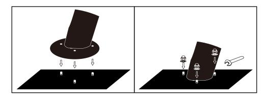
3. Find the wire joints inside the upper & bottom trunks. Connect up the joints, insert the upper trunk into the bottom one and fix the trunk with the screw preinstalled by Allen wrench.
