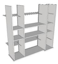
**Step 7:** Insert %" **Divider** parallel to **side**, fitting the grooves of the **Seat** and **Top Shelf**. Edge of %" **Divider** should be inserted into mortise of **Top** and **Bottom**. Repeat for remaining %" **Divider**.
