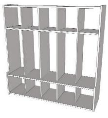
**Step 11:** Finish tightening all hex screws. DO NOT OVER TIGHTEN. Stand unit upright so that it is resting on **Bottom** panel and the edges of **Side** panels. **Assembly is complete.**
