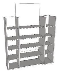
**Step 9:** Slide **Large Back** panel into the back grooves of **Seat** and **Top Shelf** until the edge rests firmly in the back groove of **Side** panel.
