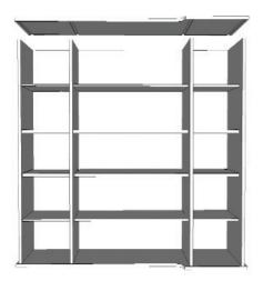
**Step 10:** Fit remaining **Side** over edges of the assembled pieces, inserting edges of **Bottom panel**, **Seat**, **Top Shelf**, and **Top** panel into mortises of **Side** panel. Make sure that back panels fit into back grooves of **Side** panel. Insert hex screws into each pre-drilled hole on **Side** panel and tighten down half way.
