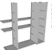
Step 5: Insert %" Divider parallel to Side, fitting the grooves of the Seat and Top Shelf. Edge of %" Divider should be inserted into mortise of Bottom. Insert hex screws into pre-drilled holes in Bottom. Tighten down half way. Repeat for remaining %" Divider.
