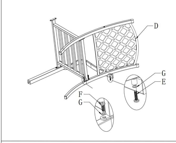
Assembly back (Part D) with the seat(Part C) according to the direction of the picture. Then put on the Part G and Screws (Part F); Put on the Part G and Screws (Part E).
