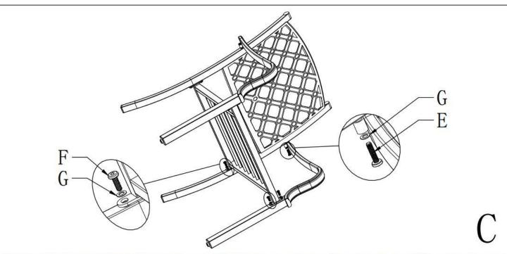
Assemble armrest (Part B) and the seat (Part C) according to the direction of the picture. Then put on the Part G and Screw(Part F). Assemble armrest (Part B) and the back(Part D) with Part G and the Screws (Part E).
