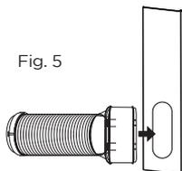
**NOTE:** The exhaust hose can be compressed or extended moderately, but it is desirable to keep the length to a minimum. Also make sure that the hose does not have any sharp bends.
