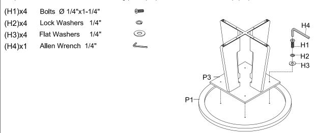
Step 4. Turn the assembled table to an upright position. Assembly is complete. **Leveler adjustment:** Levelers are pre-installed on the legs and adjust as needed to make sure the table is leveled. **Failure to follow these instructions may cause the bolts to misalign during assembly.**
