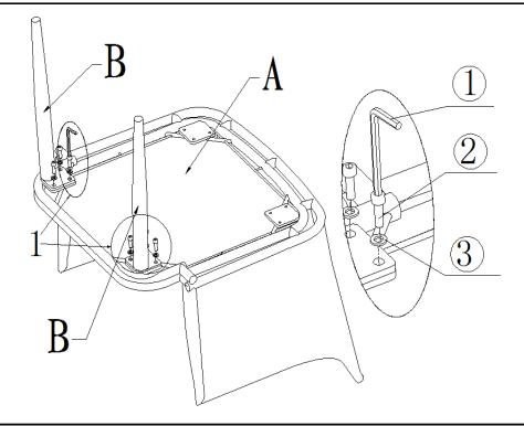
Open the carton and place all the parts onto a clean, non-marring surface. Attach Front Legs(B) to Chair Seat(A) using Bolts(2) and Washers(3) with Allen Key(1). **Do not fully tighten the Bolts.**
