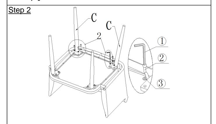
Open the carton and place all the parts onto a clean, non-marring surface. Attach Back Legs(C) to Chair Seat(A) using Bolts(②) and Washers(③) with Allen Key(①). **Do not fully tighten the Bolts.**
