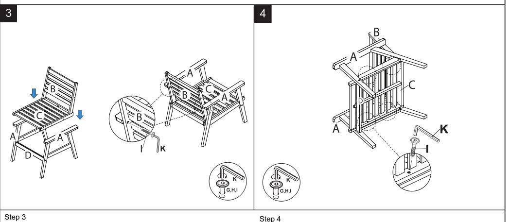
Attach leg frame (A) to back frame (B) and seat frame ,use Bolt (I), tighten with allen key(K).
