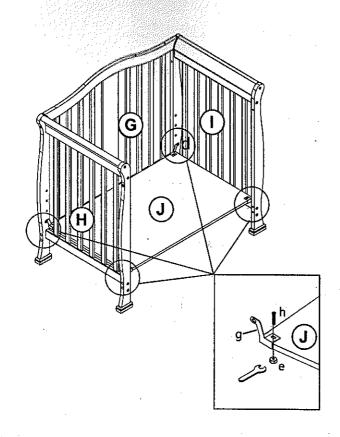
Attach metal connection(g) to the wooden mattress base(J) by using bolts(h) and nuts(e) with wrench. Position the wooden mattress base (J) to a selected position on legs. Insert the bolts(d) into thread inserts on legs,then tighten securely with Allen wrench(i). Be sure the flat side of wooden mattress base(J) is upward.
