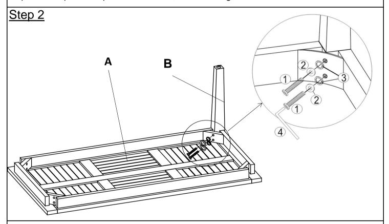
Attach Leg (B) to Table Top (A) by using Bolt (1), Flat Washer (2), Spring Washer (3) with Allen Key (4)
