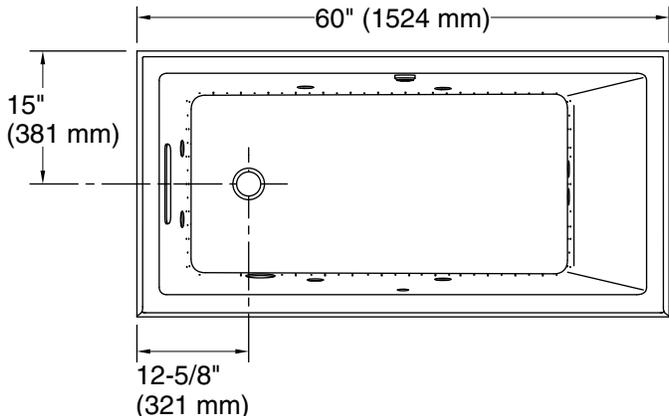
No change in measurements if connected with drain illustrated. (K-7271)
