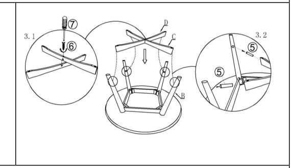
First, fix the connecting rods (C) and (D) with a screwdriver (7) and Rapid tooth (6), as shown in Figure (3.1). The wooden tenon (5) is inserted into the connecting rod (C) (D) and the table leg (B), as shown in Figure (3.2).
