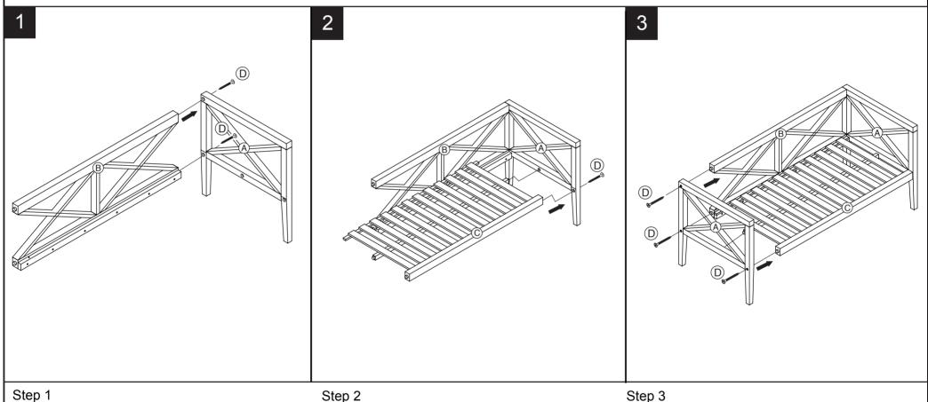
Attached back frame (B) to (A). Using Screw (D) tighten by (E).
