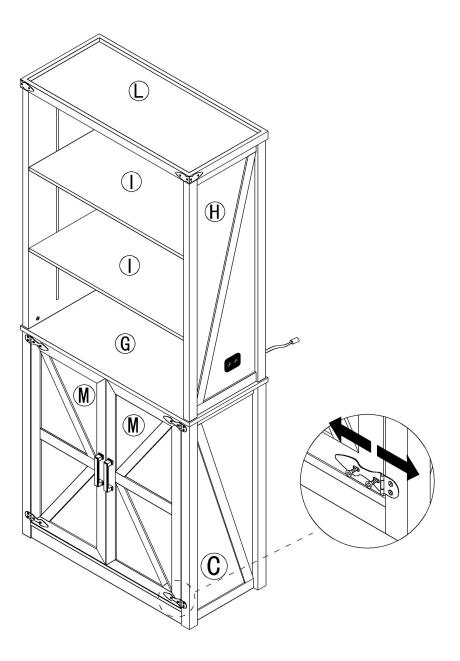
If there is a large gap after the installation of the door, please twist the screw of the door hinge back halfway and move the door left and right.
