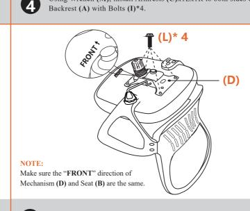
Using Wrench (M), attach Mechanism (D) (6)to the Seat (B) with Bolts (L)\*4.
