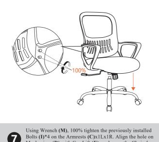
Using Wrench (**M**), 100% tighten the previously installed Bolts (**I**)\*4 on the Armrests (**C**)x1Lx1R. Align the hole on Mechanism (D) with Gas Lift (E), and press the Chair down until it is fully secured.
