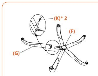
Turn the Base (F) upside down, insert the Legs (G)\*5 into the Base one by one. Use Wrench (M), secure both with Bolts (K)\*10. (1)
