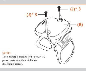
Turn the Seat (B) upside down . Using Wrench (M), install Armrests (C)x1Lx1R to the Seat with Bolts (J)\*6.
