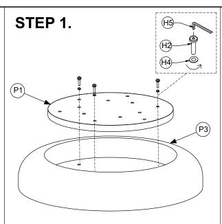
\*Screw the bolts out to take frame out (P1) of top (P3)
