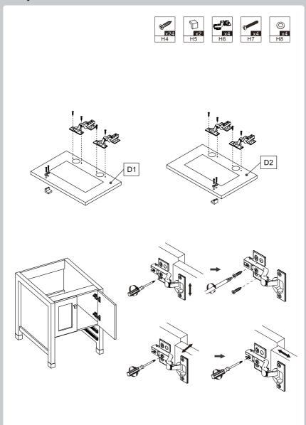
Adjust the screws as shown on the sketch map to ensure all the door gaps are in the same level.
