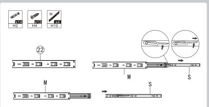
Keep pressing here, then pull out to devide the slide.
