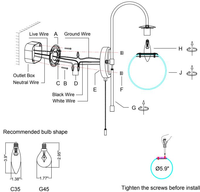
Max. Size of Bulb: 1.77 Inches Wide \* 3.94 Inches High Tighten the screws before installing the glass globe. Note: Do not over tighten the screws or you will potentially break the glass.
