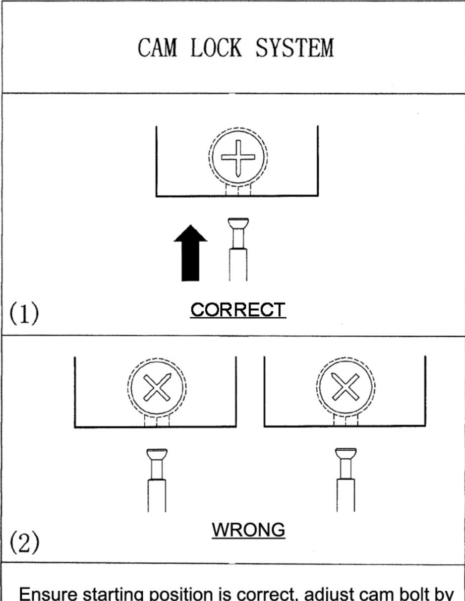
Ensure starting position is correct, adjust cam bolt by pushing or pulling during assembly. Turn clockwise until secure.
