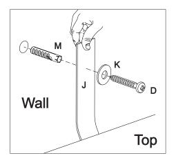
With drilling machine make one hole in the wall, Insert part (M) in the hole.
