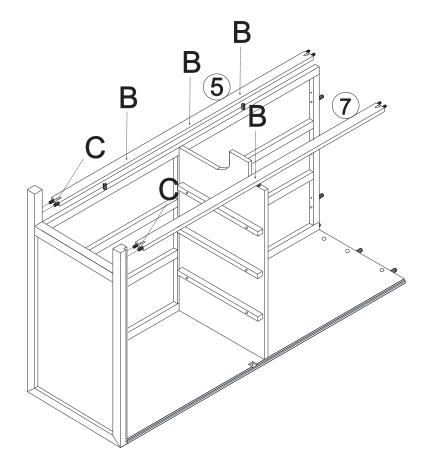
Step 8 Insert screw B (x3), C (X2) Cam lock D (x3) into parts (3).
