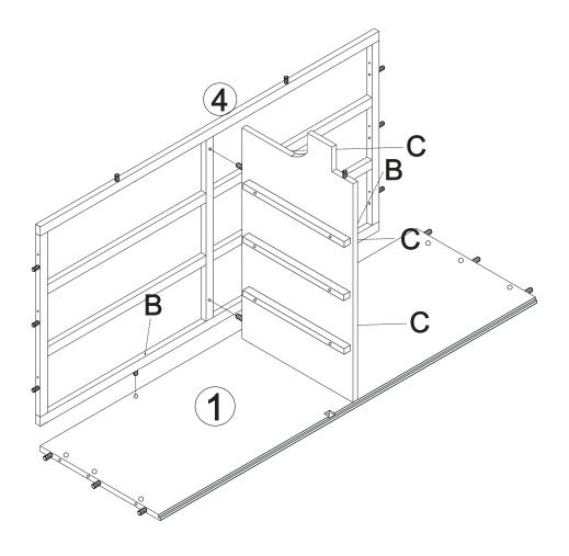
Step 6 Insert screw B (x3) Cam lock D (x3) into parts (2),(1).
