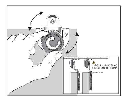
Slide the door close to the door jamb. If there is a gap between the door and the door jamb, rotate the plastic gear until the gap is eliminated.
