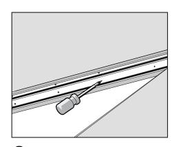
Attach track to the head jamb with longer screws (4.2mmx32mm)
