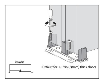
Slide the door close to one door jamb and install the floor guide and secure with screws(4.2mmx 19mm)
