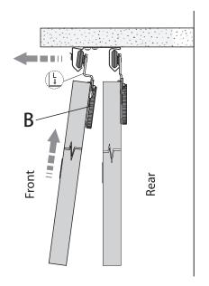
Later hang the door attached with **B type** roller(L-SHAPED) to the **front track** with 20 degree angle.
