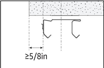
Center the track on the head jamb if the opening is deep enough; otherwise, ensure a 5/8-inch gap from the jamb edge to the outer side of the track and mark holes with pencil.
