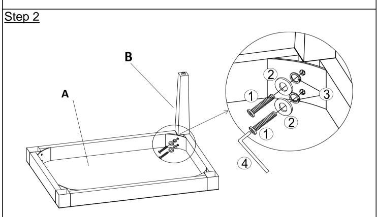
Attach Leg (B) to Top (A) by using Bolts (1), Flat Washer (2), Spring Washer (3) with Allen Key (4).
