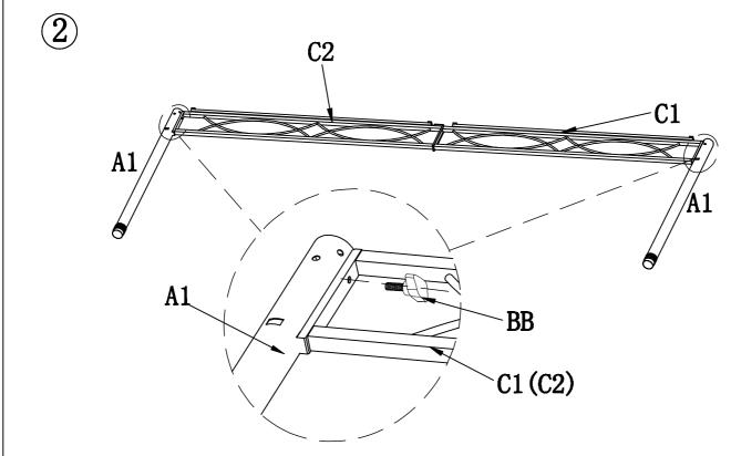
STEP 2: Attach Upper post (A1) to assembed Cross Beam (C1,C2), then fix by using screw (BB)
