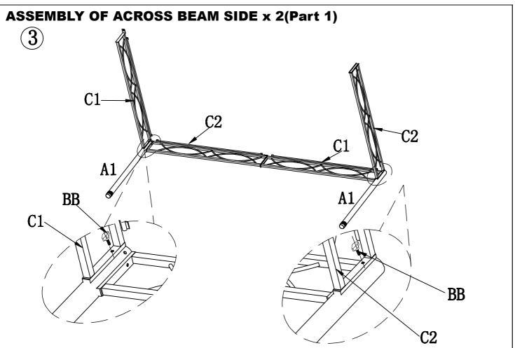
Step 3: Attach Across Beam (C1,C2) to Upper Post (A1), then fix by using Screw (BB)
