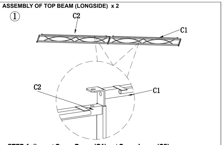
STEP 1: Connect Cross Beam (C1) and Cross beam (C2).
