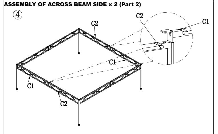
Step 4: Connect Side Across Beam (C1) and side across beam (C2).
