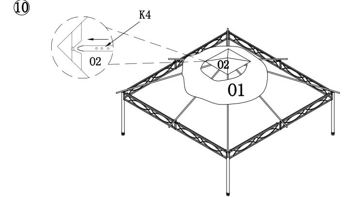
**Step 10:** Put **Small Canopy (02)** on small roof frame, fix four corner to **Small Roof Extension Tube (K4)**, then adjust the tube length make canopy fitted.
