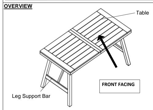
This Table has multiple parts and may require up to some 30 minutes to assemble. To give you an overview of the Table parts, the above picture is to help you put the various parts into perspective. Please read through the instructions below to familiarise yourself with the parts and steps before assembly.
