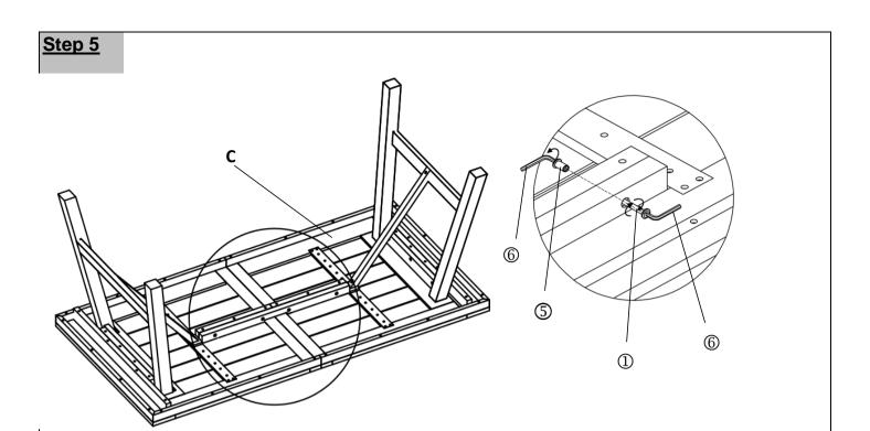
Position Middle Support Bar(C) as shown in picture above.
