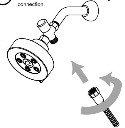
5 Thread Hose end marked "HAND SHOWER" onto base of Handheld Shower. Hand tighten connection.
