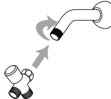
3 Thread fixed Showerhead onto front outlet of Diverter. Tighten with Adjustable Wrench.
