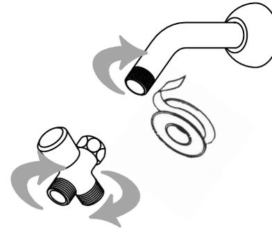
2 NOTE: Inspect Diverter to be sure Sealing Washer is in place within Coupling Nut.
