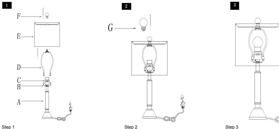
Step 1 Insert the Harp (D) into the Saddle (B). Put the shade(E) on the Harp(D), then tighten the Finial (F)into the Harp (D)
