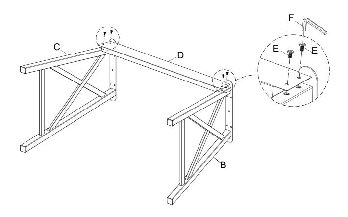
2 Attach Left Side Frame (B), Right Side Frame (C) and Back Apron (D) to Top Panel (A) using Bolt (E) by Allen Key (F) as below shown.
