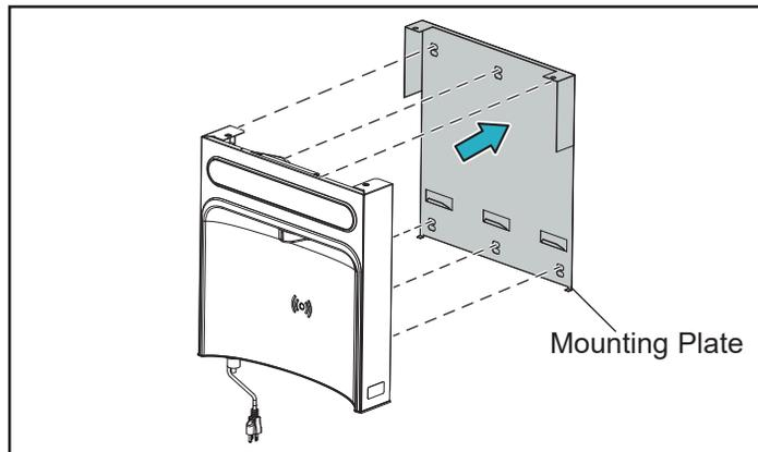
3. Place mounting plate against wall on top of the basin. Center the mounting plate side to side with the basin. Mark the six (6) mounting holes with a pencil.
