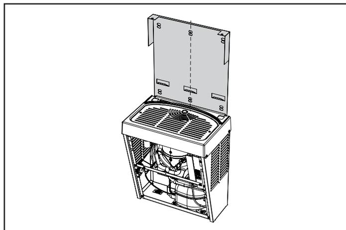
4. Install the wall mounting plate to the wall using six (6) 7/16" screws through the mounting holes. Use appropriate fasteners for your wall type.
