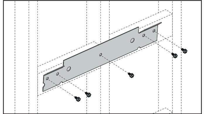
4. Hang unit onto the hanger bracket.
