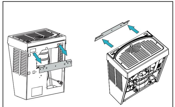
5. Install the two mounting screws to attach cooler to the wall.
