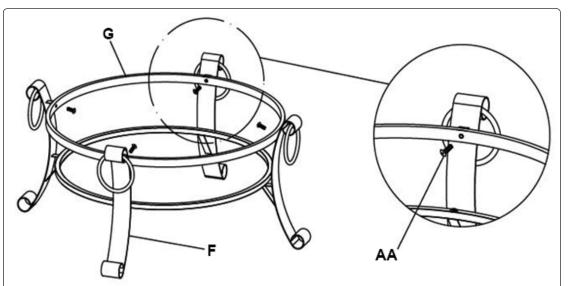
Step 3: Connect Upper Support Ring (G) to the legs (F) by using M6x16mm Bolt (AA). Tighten all the hardware.
