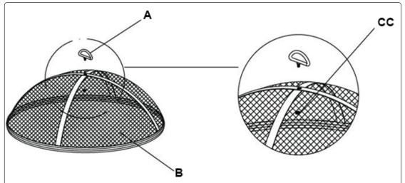
Step 1: Insert handle (A) into hole in Safety Mesh Screen (B) and tighten it with M6 Nut (CC) underside to secure.
