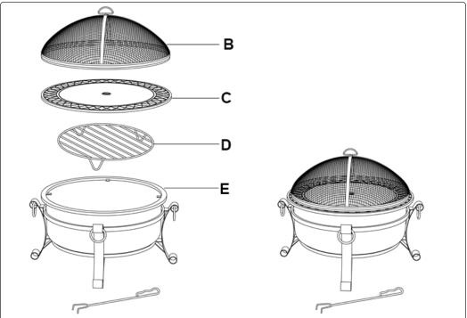
**Step 5:** Place the wood grate (D) into the fire bowl (E) and put the tabletop lid (C) on the fire bowl, then place safety mesh screen (B) onto the tabletop lid. Finally place the poker (I) near the base assembly.
