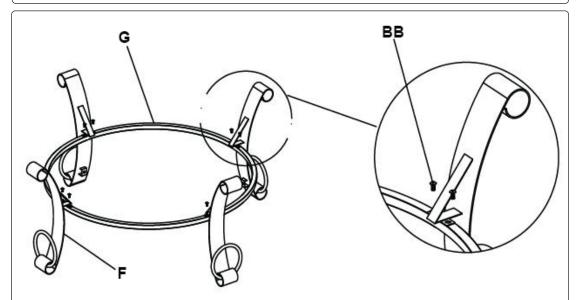
**Step 2:** Connect Lower Support Ring (H) to the legs (F) by using M6x12mm Bolt (BB), Do not tighten hardware at this time.
