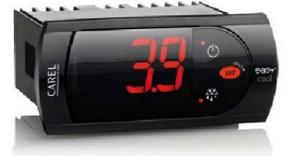
To turn the unit **ON/OFF**, press **UP** for more than 3 seconds. The control and defrost algorithms are now disabled and the display will read **OFF** alternating with the current temperature inside the unit as measured by the temp sensor. To engage the manual defrost, hold the **DOWN** button for more than 3 seconds. It will still show the current temperature.
