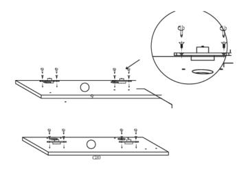
• Apply the screws to fix the hinges on the shelves G 10.
