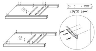
• Insert the screws to connect the slides (N-1) to the shelves.
