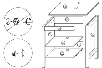
• Install shelves G6, G7, G8 in order. Then tighten the cam lock with the cover.
