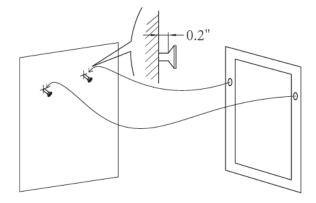
Insert the expansion into the anchor. Leave about 5mm (0.2") clearance for the mirror. Then connect the mirror.
