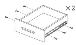
$\bullet$  Insert the screws to conncet the slides(M-2) to the drawer side.
