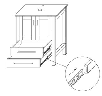
• Connect the drawer to the slide inside the cabinet. Then slide the drawer in and out to ensure smooth operation.
