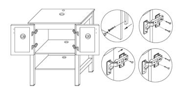
Use E SCREWS to connect the hinge bracket to the cabinet.
