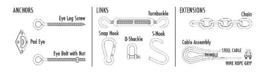
There is an extensive range of fixing accessories available to help you secure your shade sail(s). Chain, wire, or thick strong rope can be used to extend your shade sail corner to a fixing point if required.
