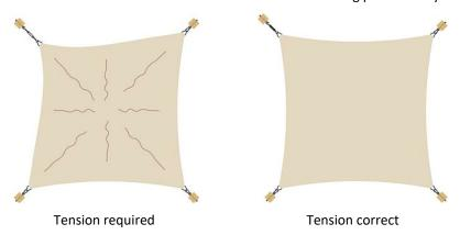
A properly mounted and tensioned shade sail will have approximately 100 pounds of tension on it and will have few to no wrinkles. Connect all points, using rope or wire cable if necessary, to gain increased leverage. The rope can be threaded around a number of times so that it works as a "pulley" mechanism. Another tensioning method would be to use a turnbuckle which can aid in applying the proper amount of tension. Stop tensioning when the shade sail is rigid with few or no creases.
