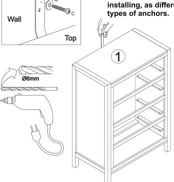
With drilling machine make one hole in the wall, Insert part (M) in the hole.
