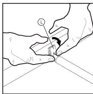
3.Put the plastic clamp(L) into the lower part of hole on 45degree.
