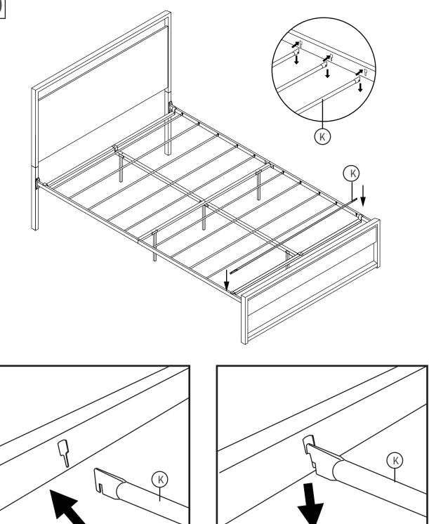
1. Insert slats into the hole 2. Push the slats into the gaps. on sidebar in the correct orientation.
