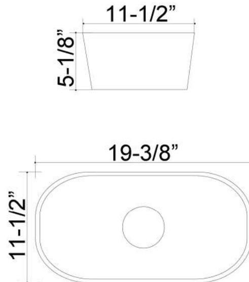
Dimensions of fixture are nominal and may vary within the range of tolerances established by AMSE Standard A112.19.2.2013 Dimensions and specifications subject to change without notice.
